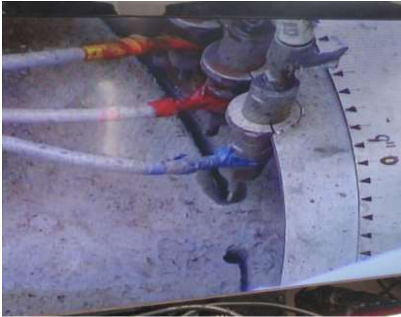
Above Left: Olivine or garnet/water jet cutting method.
