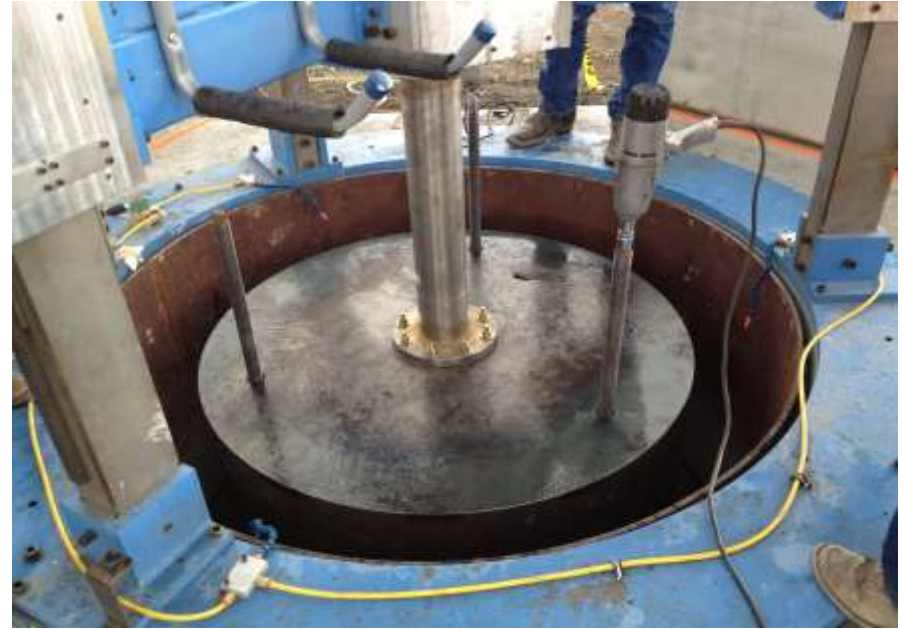
Above Right: Rotary cutting method.
