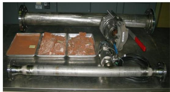
**Figure 3.** Unexpected Simulated Sludge Buildup in Process Piping
